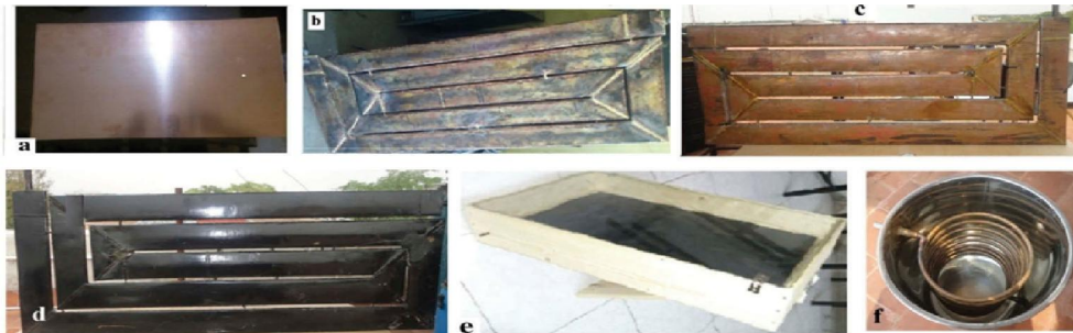
Figure 1. Fabrication process of the system. (a) Copper Sheet of Dimension. (b) Absorber through welding process. (c) Absorber after welding process is complete. (d) Black coated absorber. (e) Wooden box with insulation. (f) Storage tank with heat exchanger.
