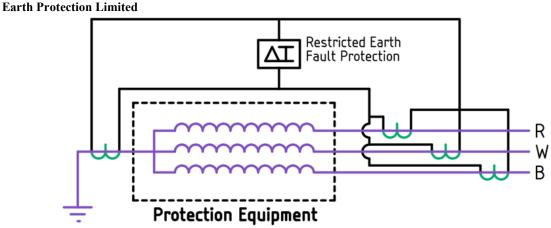
When the transformer fails, a large amount of fault water will flow. In this case, the fault must be repaired as soon as possible. The ability to act on a protection must be limited to the area of the transformer; This means that if a ground fault occurs in a different location, the relay must be sent to the area where it should be, while the other relays must remain unchanged. That is why this relay is called limited earth fault protection relay.
