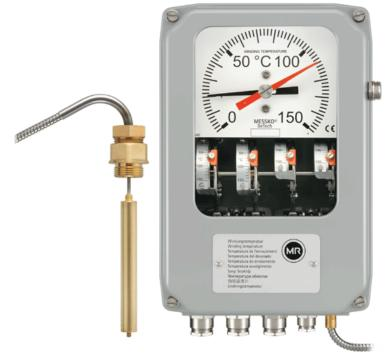
On the box there is an indicator dial (black pointer) that shows the temperature of the transformer and a red pointer that shows the alarm light spot. If the black pin exceeds the red pin, the device will activate the alarm. Looking at the bottom, we can see four arrows with which we can set the device for alarm or motion, or use it to start or stop the pump or cooling fan.
