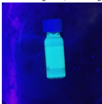
Fig2: Fluorescence of carbon dot observed in UV Chamber
