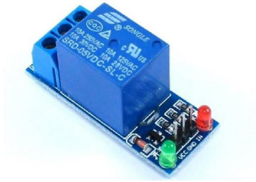
Fig: Relay Switch
