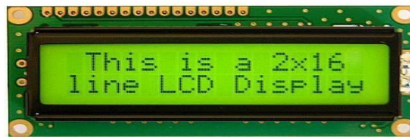
Figure 5: 2x16 LCD Display
