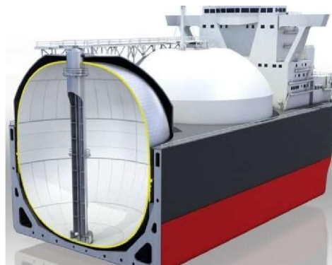
Figure 1. A marine LNG tank and its cut view
