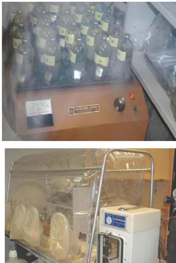
Figure 1: (top) anaerobic chamber; (bottom) sediment bottles on platform shaker
