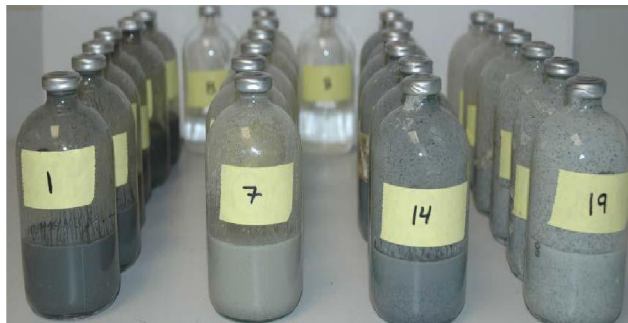
Figure 3: Photograph of microcosm bottles after 2 months of incubation (1st row: Mesteña sediments amended with H 2 ; 2nd row: Mesteña sediments amended with acetate; 3rd row: URI sediments amended with H 2 ; 4th row: URI sediments amended with acetate; control bottles with only groundwater are at back).
