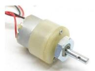
DC Motor -300RPM -12Volts geared motors are generally a simple DC motor with a gearbox attached to it. This can be used in all-terrain robots and variety of robotic applications. These motors have a 3 mm threaded drill hole in the middle of the shaft thus making it simple to connect it to the wheels or any other mechanical assembly.
