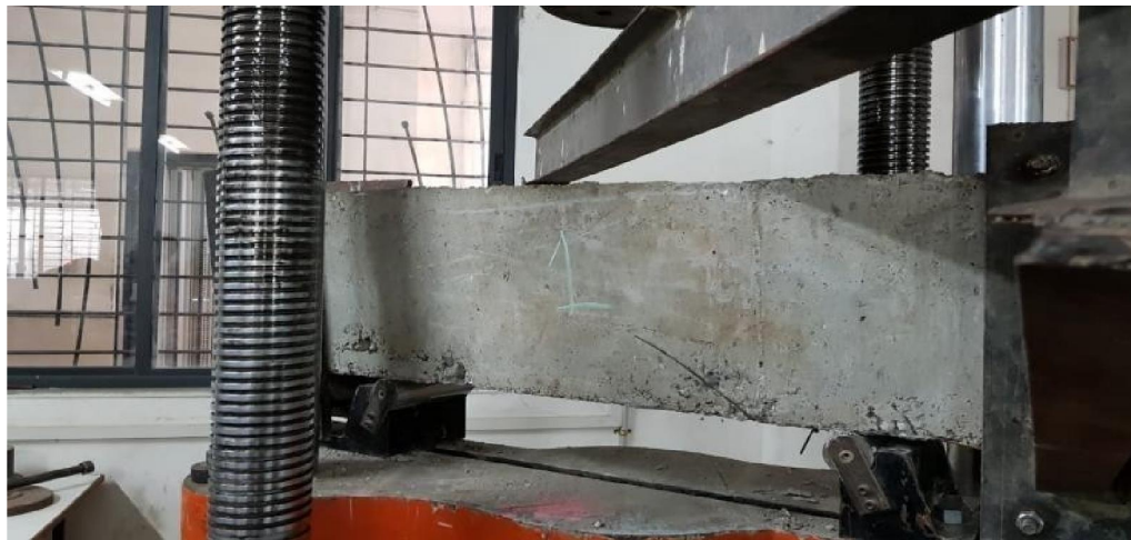
Figure 3: Experimental setup of the control beam
