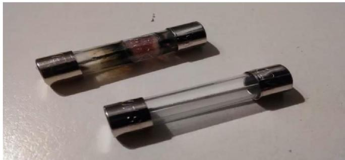
**Figure 1:** The microwave fuse has blown due to overheating.
