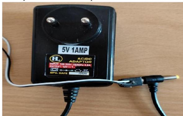
**Figure 7:** 5V 1A power adapter
