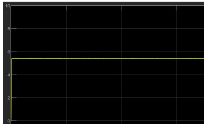
Fig 6: Output voltage of the rectifier
