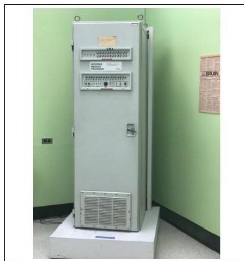
Figure 2: First ARPANET Router [11]
