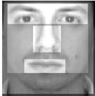
Figure 5.3 face recognition using template matching
