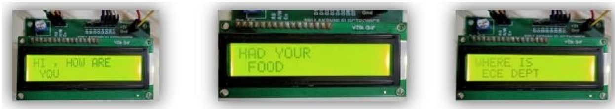
Fig 4.2 Messages from flex sensors
