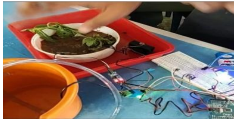
Fig 7. Two glowing lights indicatesoil is moist enough and no water flows.
