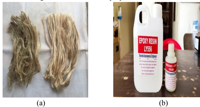
Figure 1: a) raw banyan and banana fibers. b) The Hardener (HY951) and epoxy resin (LY556)
