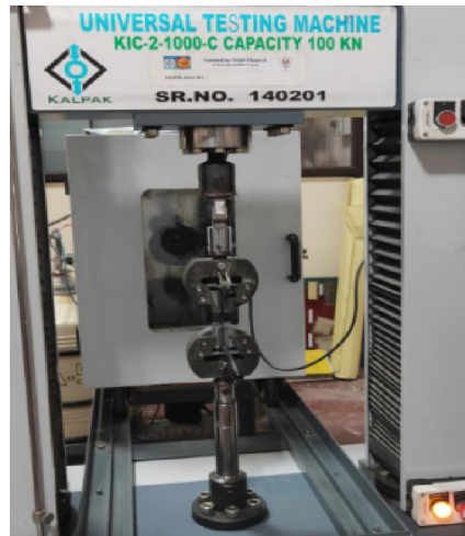
Figure 3: Tensile test experimental setup
