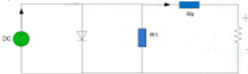
Fig. 2 Equivalent model of solar cell
