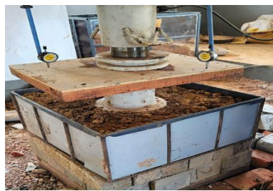
Fig.12 Settlement Analysis using Plate load Apparatus
