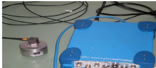
Figure 9. Piston Specimen with Accelerometer and FFT analyzer
