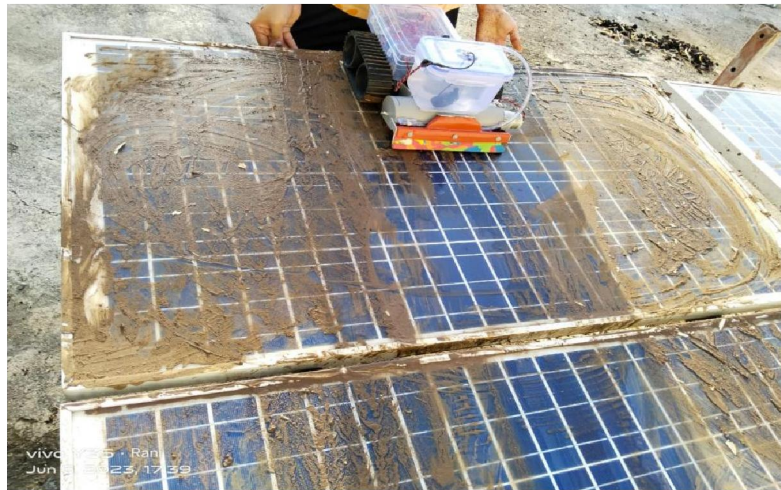
Fig. C Cleaning Processing of Solar Panel
