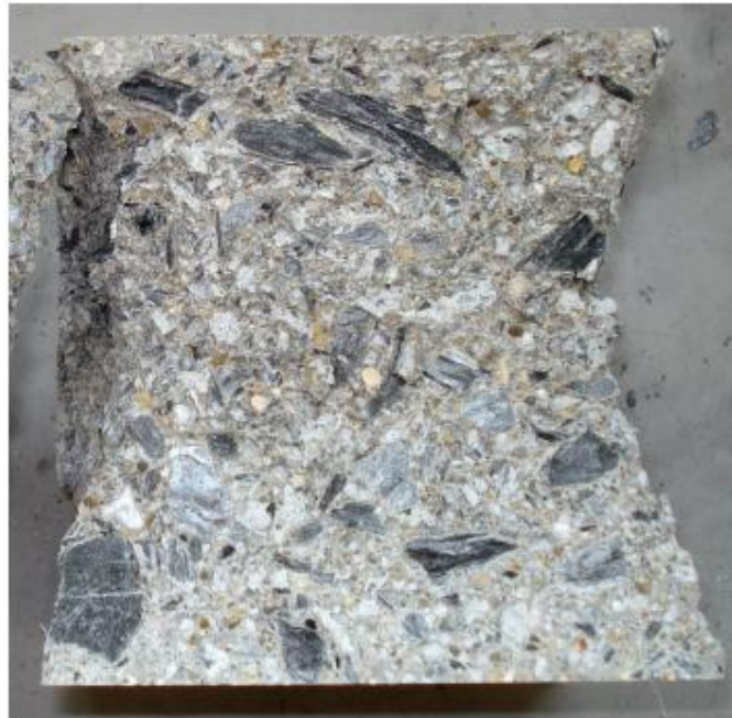
Figure 5- Concrete cube test specimen after compressive strength testing
