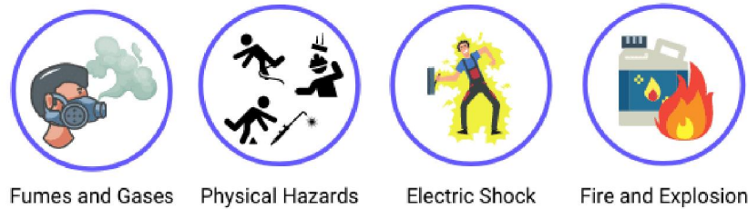
Figure 1. Welding and Cutting Hazard
