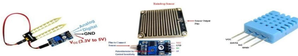
Figure-2 Soil Moisture sensor Figure – 3 Raindrop sensor Figure-4 Temperature & Humidity sensor Smart agriculture system
