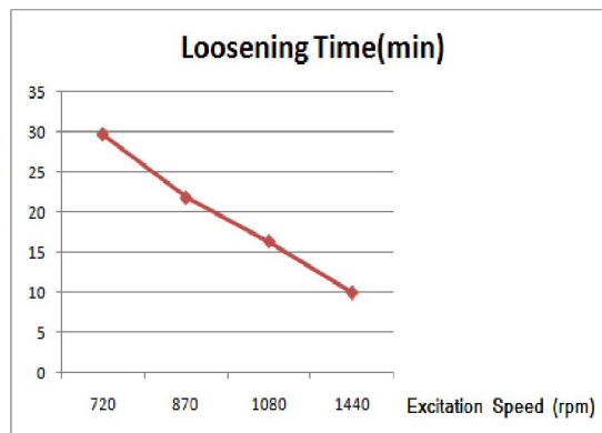
Graph of Loosening time Vs Excitation Speed (spring washer)
