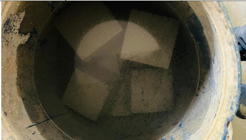
Picture no. 1: curing of concrete cube in distilled water
