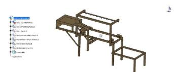
Supporting frame fabricated with Steel angle section 30x30x3mm. Which supports the complete setup including water tanks at bottom. A supporting provision is provided with frame for barrel open end to avoid vegetables fell out of the barrel during cleaning. Height of setup is 1524mm.
