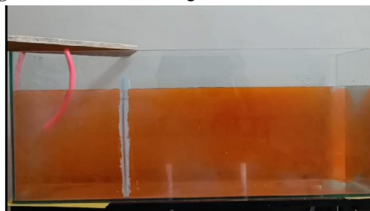
Fig. 9: Water model of single strand tundish without dam.
