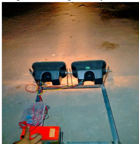
Fig. 4: Automatic Headlight Dipper System
