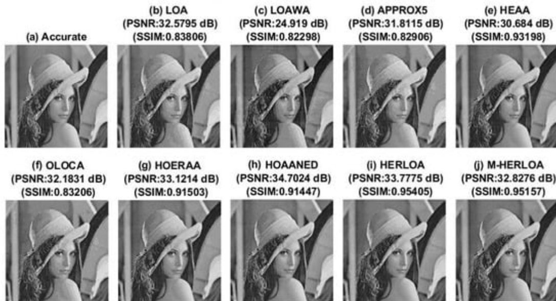
Figure 2. Image processing result for ‘lena’ image obtained using accurate and approximate adders:
