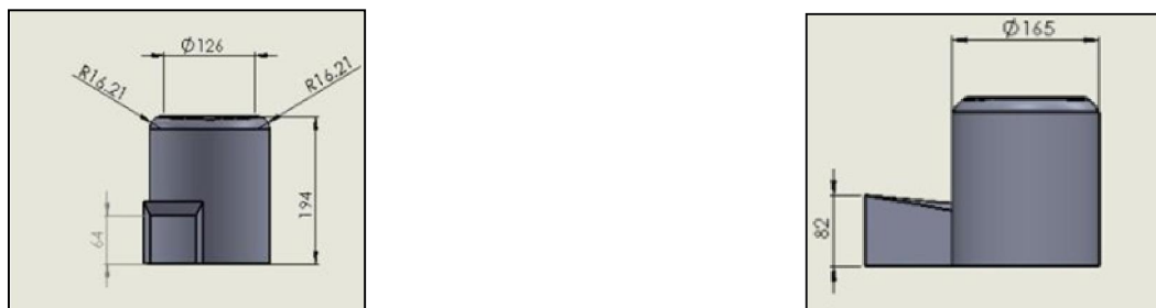
Figure 4: (a) Front View of Cook stove (b) Left hand side view of Cook stove
