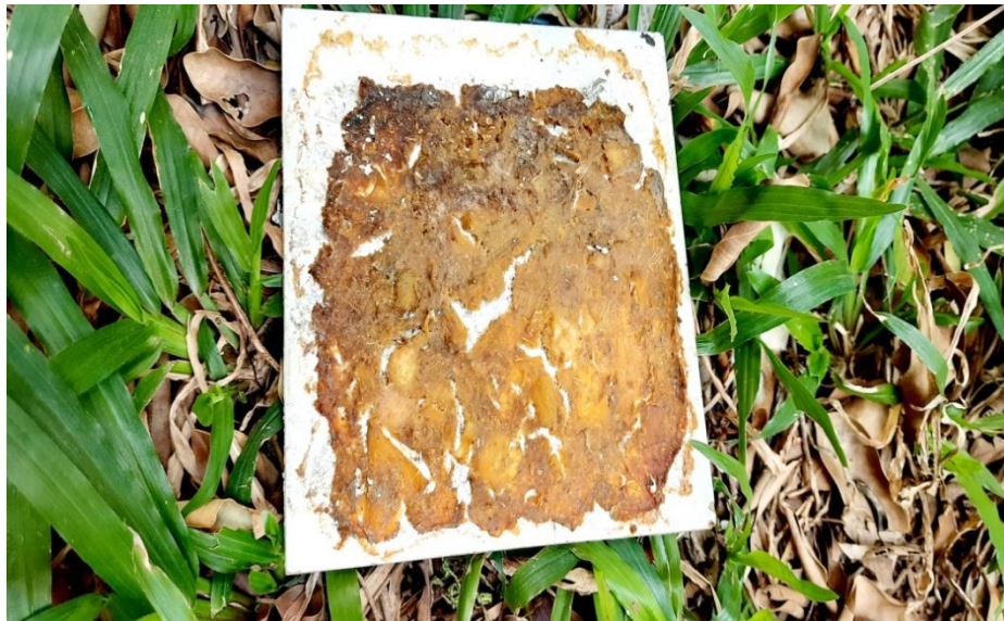
Figure 15 – Bioplastic formed from the fruit peels
