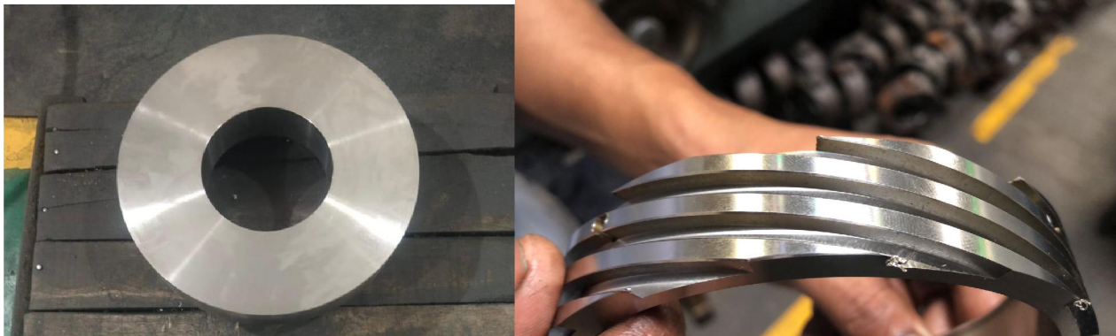
Fig. Pumping ring (manufactured using 5 Axes VMC)
