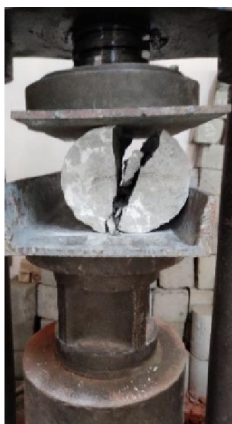
Fig. No. 3.1: Compression & Split Tensile Strength Test on CTM Fig. No. 3.2: Flexural Strength Test on UTM
