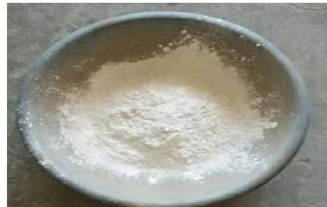
Fig. No. 2.2: Ceramic Waste Powder
