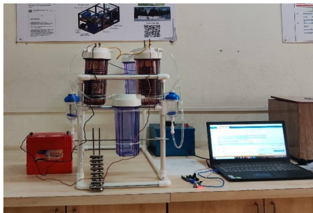
Fig -08: Actual Setup of Efficient Hydrogen Electrolysis System
