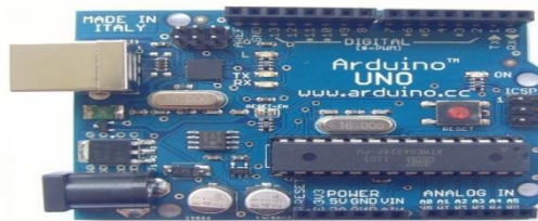
Figure 1:-Arduino with ATmega328P microcontroller
