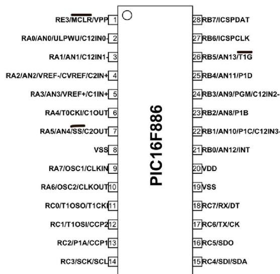
Fig. 4. PIC 16f886 microcontroller
