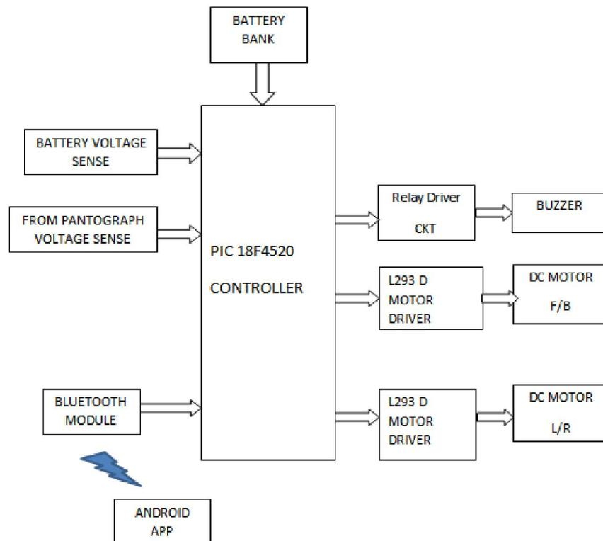
Fig. 1. Block Diagram (Vehicle unit)
