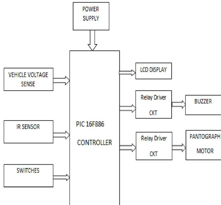
Fig. 2. Block Diagram (Charging Station unit)
