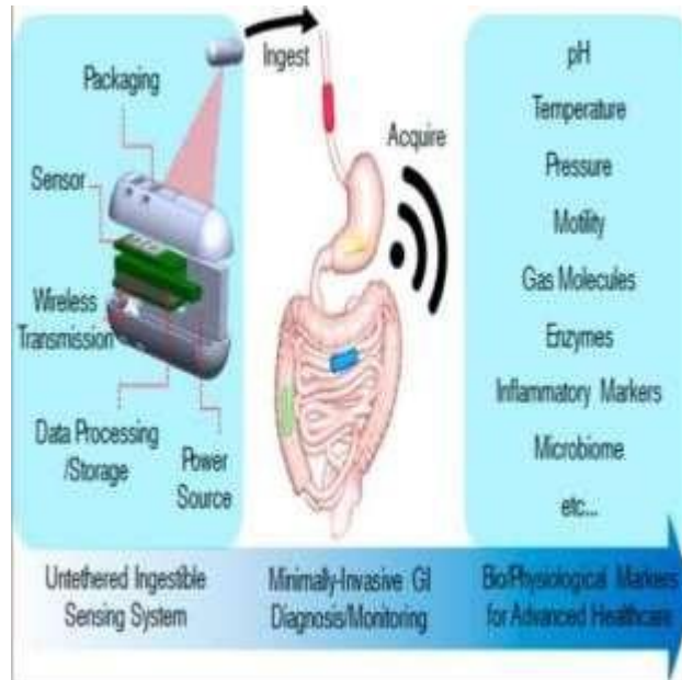
Fig 2. block diagram of ingestible sensor in health care
