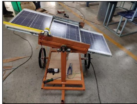
Fig. 3. Inclination of panel assembly to demonstrate sun tracking
