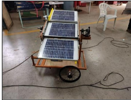
Fig. 2. Panel assembly in an unfolded position
