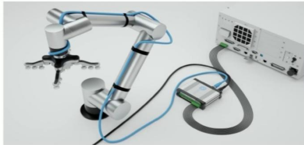
Fig3: Electrical connections of gripper
