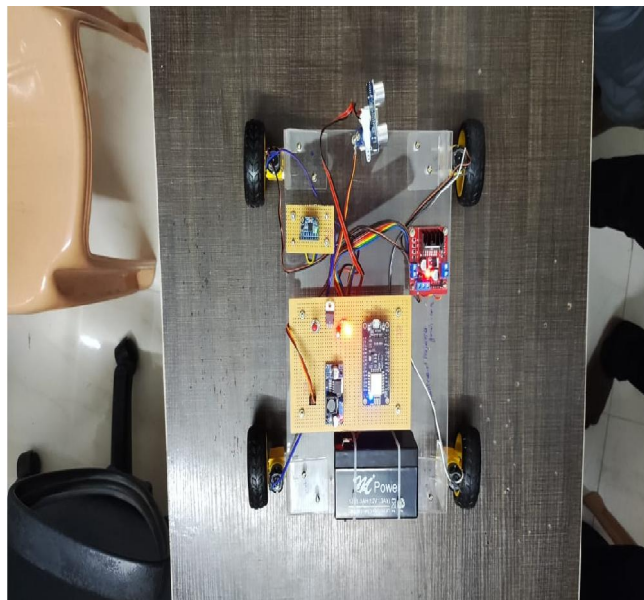
Fig 6.1: Robot with Obstacle Detection
