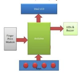
Whenever user place his finger over fingerprint module then fingerprint module captures finger image, and search if any ID is associated with this fingerprint in the system. If fingerprint ID is detected then LCD will show Attendance registered and in the same time buzzer will beep once and LED will turn off until the system is ready to take input again.
