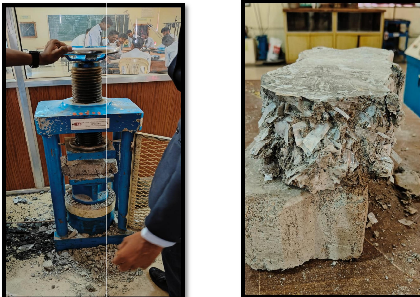
Fig1 . Paving block Testing
