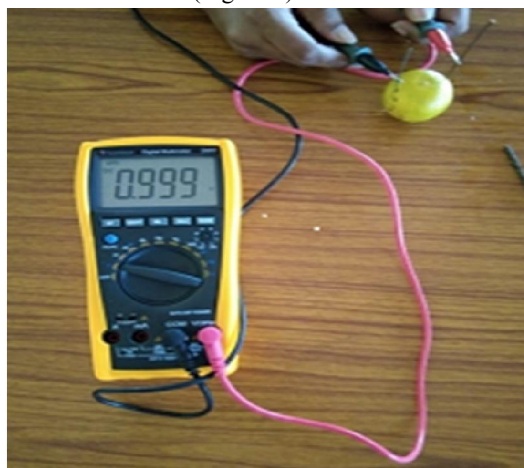
Figure 1: Experimental setup and measurement of voltage
