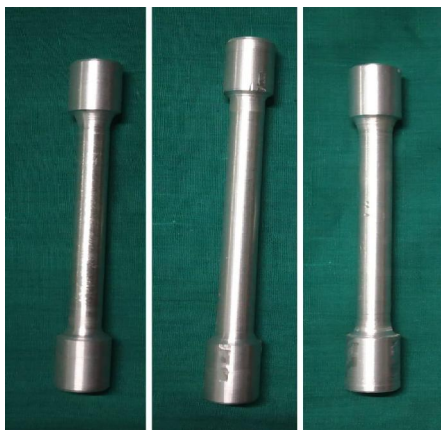
Fig 6: Tensile specimen before testing
