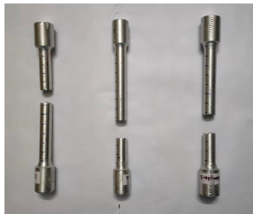
Fig 7: Tensile specimen after testing
