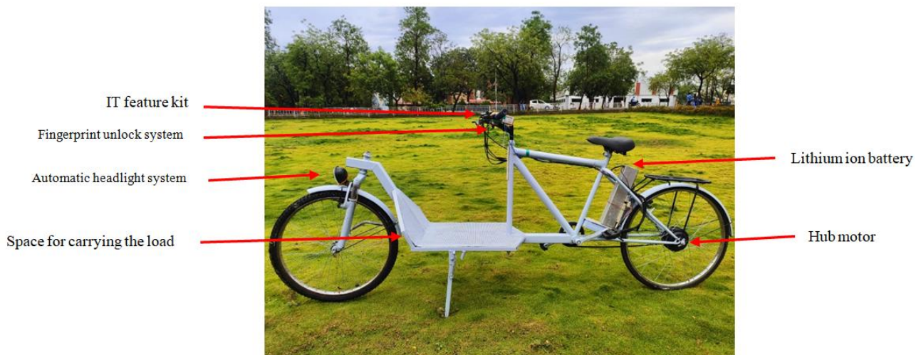
Fig.11.Design and development of E-cargo bicycle
