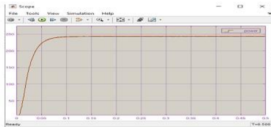
Figure 7 (c): Power of PV panel using ANN MPPT controller applied to the boost converter under fixed weather conditions ( R=1000\text{W/m}^2, T=25\text{deg C} ).
