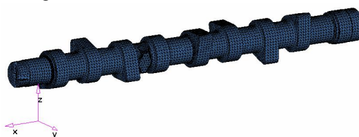
Fig. 3: A 3-D plot with meshing of the camshaft used for a specific engine
