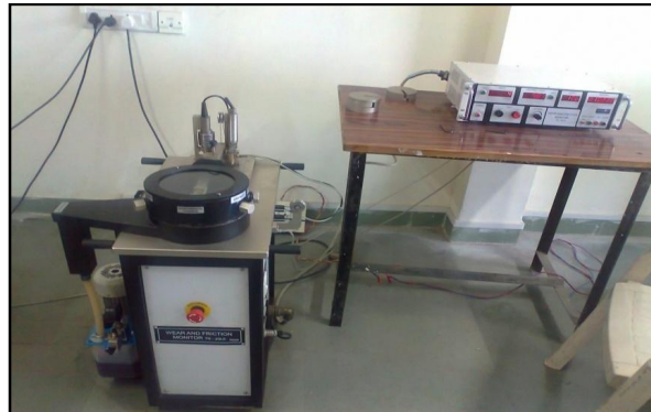
Figure 5: Photograph of experimental set up (Tribometer TR-20LE).
