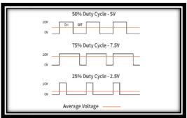
The DC motor acts as a low-pass device (rejects high frequency harmonics) and has a speed proportional to the DC value of the applied voltage. So, if the PWM frequency is high enough, what the motor "sees" in the applied PWM is that average value, or DC value. And adjusts its speed accordingly
