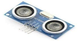
The sensor emits a burst of ultrasonic waves, typically in the range of 40 kHz to 200 kHz. These sound waves travel through the air and, when they encounter an object, they bounce back or get reflected.
