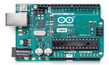
The Arduino Uno board features digital input/output pins, analog input pins, PWM (Pulse Width Modulation) outputs, UART (Universal Asynchronous Receiver-Transmitter) for serial communication, and various other interfaces. It also has a USB connection for programming and power supply.
