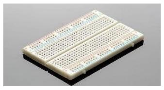
A breadboard, also known as a protoboard or solderless breadboard, is a device used to create and test electronic circuits without the need for soldering. It provides a platform for quickly and easily connecting electronic components, such as resistors, capacitors, integrated circuits, and wires, for rapid prototyping and experimentation.
