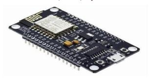
The Node MCU board is designed to be programmer-friendly, allowing developers to easily program and interact with it using the Lua scripting language or the Arduino IDE. It has a USB interface for power supply and programming, as well as a set of general-purpose input/output (GPIO) pins for connecting and controlling external devices.
